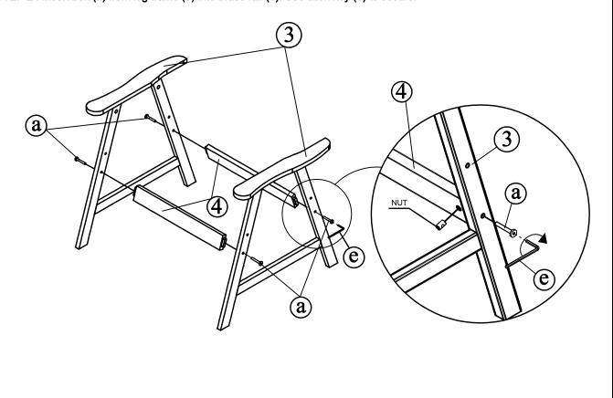
STEP 3 : Attach the frame in step 1 to the frame in step 2.
